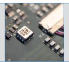
The electronic levelling system compensates for unevenness in the set-up area and is thus an absolute highlight of the MLT 3000. A deviation of only a few millimeters already results in an incorrect assessment of the measurement results. The deviations detected by the position sensor are automatically compensated by the MLT 3000 software, thus avoiding incorrect measurements.
