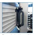
The vertical guidance of the light collecting box is maintenance-free and runs particularly smoothly thanks to the ball bearing guide rollers.
