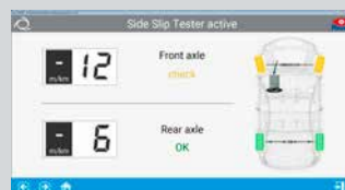
Side slip test Clear display of the directional stability of the vehicle axes.
