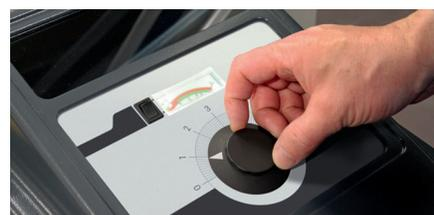
Mechanical height adjustment enables the projection screen to be moved vertically in the housing. The hand wheel fitted with a scale can be used to preset the required inclination angle for the headlight.
