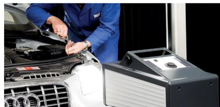
The headlights are aligned via the projection screen that is visible from the side of the vehicle. Border lines printed on the screen are used to compare the actual value with the target value and facilitate alignment. A deflection mirror makes the headlight projection visible from the front of the unit as well.
