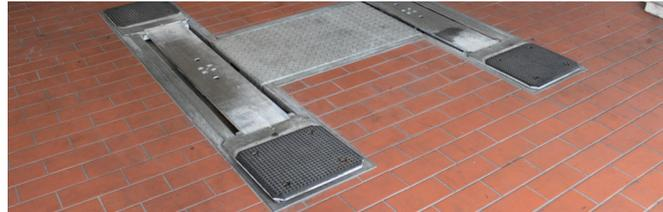
For easy driving over the flat head support. The D-ER mounting frame (VZ 972420) and the straight extensions (VZ 972519) help to install the flat head lift in a flush-mounted manner. This ensures quick lifting and lowering without adjusting the extensions.
