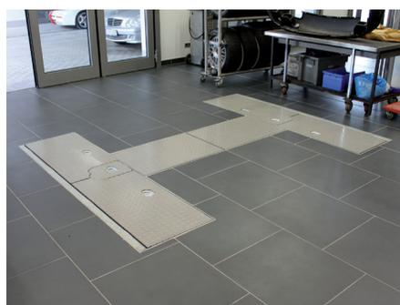
Fully covered swing arm support, traversable with 2 t wheel load
