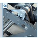
Maintenance-free cylinder raising support: full lifting capacity is effective at lower heights already. Smooth pick-up and lowering of load with reduced speed.
