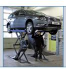
The generous lifting height allows comfortable working even with flush-floor installation.
