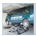
Very long extension length of the support plates (1550 - 2100 mm), making lifting of smaller vans possible.
